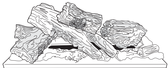
Figure 42a. Incorrect Log Position.
